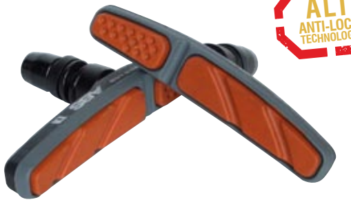
ALT-02V V Type-Hybrid-MTB 72mm ALT ANTI-LOCK-TECHNOLOGY Brake Pad Controlled Braking. Dual density rubber combination offers, anti-lock braking function, Shorter braking distances, Shimano system compatible, Better braking power control
